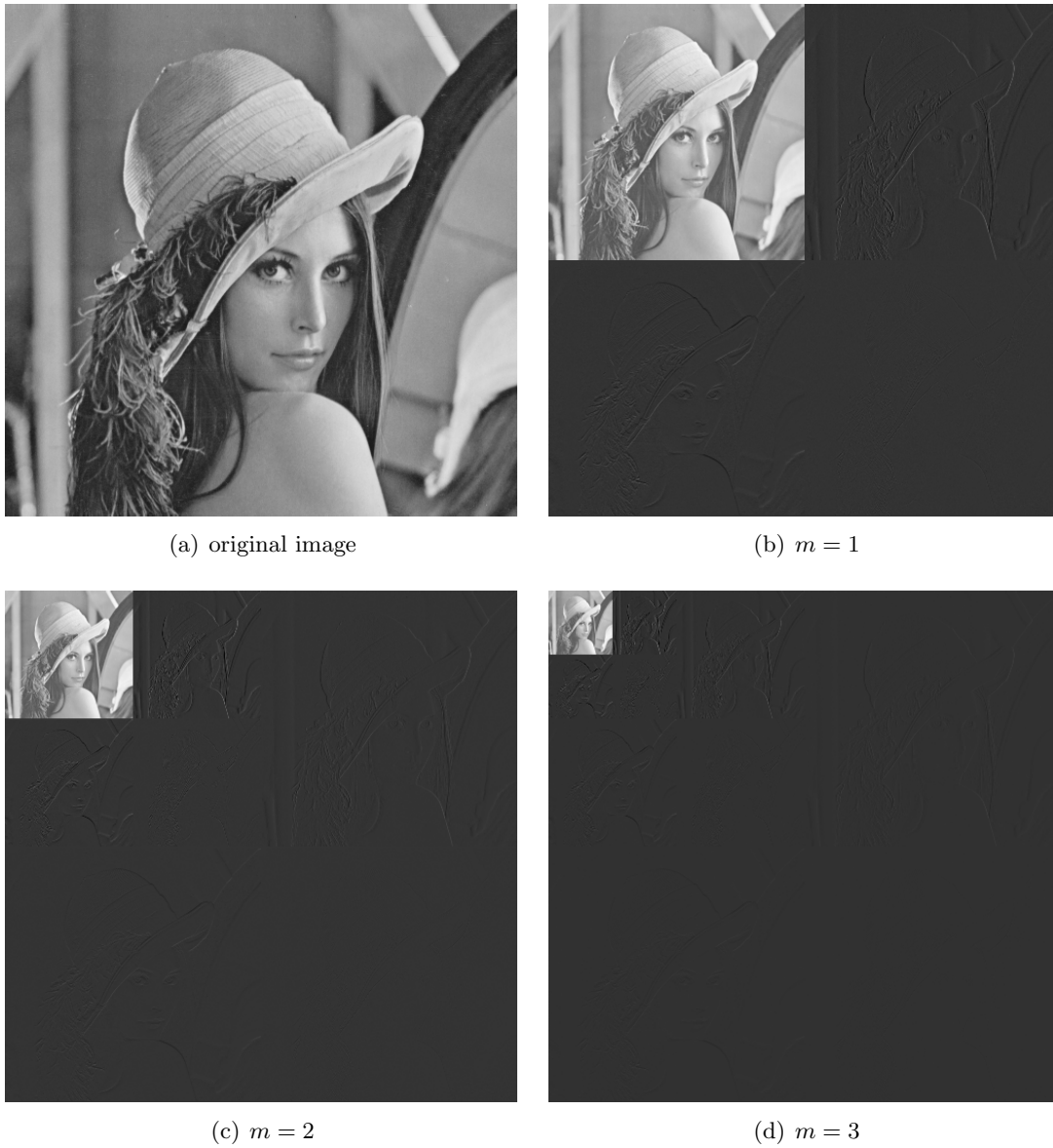
Figure 3.7: The figure shows the m -level DWT of the Lena image for various values of m .
