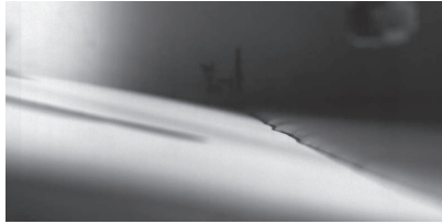
FIG. 7. Image showing part of the shoreline before start of runup, with water to the right. The front of the wave has reached the shoreline, but it has not yet been set into motion.
