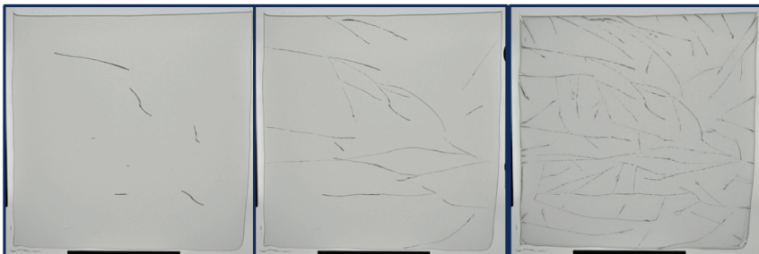
Figure 14: Time development of fracture network in gelatine experiment.
