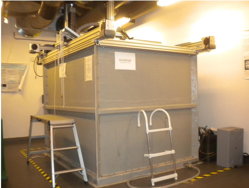
Figure 4.2: Water tank at the sonar laboratory with the dynamic position system mounted on top
