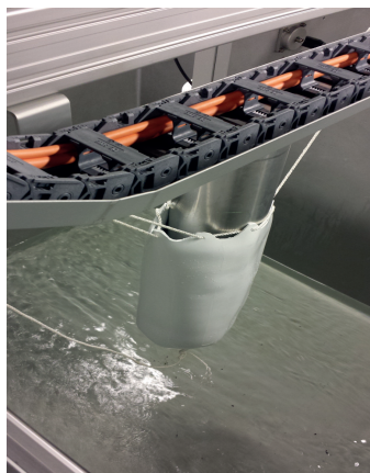
Figure 5.10: The transducer covered by the fender
