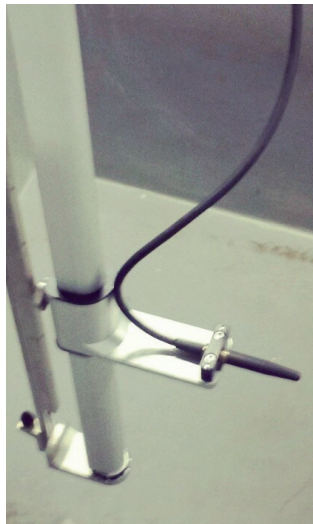
Figure 5.11: The hydrophone, Teledyne Reson TC4034
