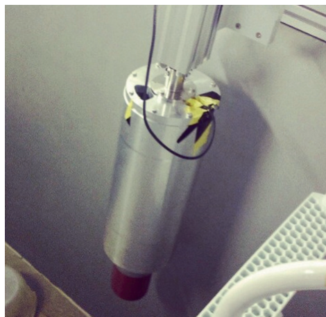
Figure 5.6: The transducer, Simrad SH90 mounted on the bottom of the tube.
