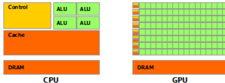
Figure 2.1: An overview of the CPU and the GPU architecture. As seen, the CPU devotes more of its transistors to cache and control logic, while the GPU dedicates most of its transistors to arithmetic units. Original figure from CUDA C Programming Guide [28].
