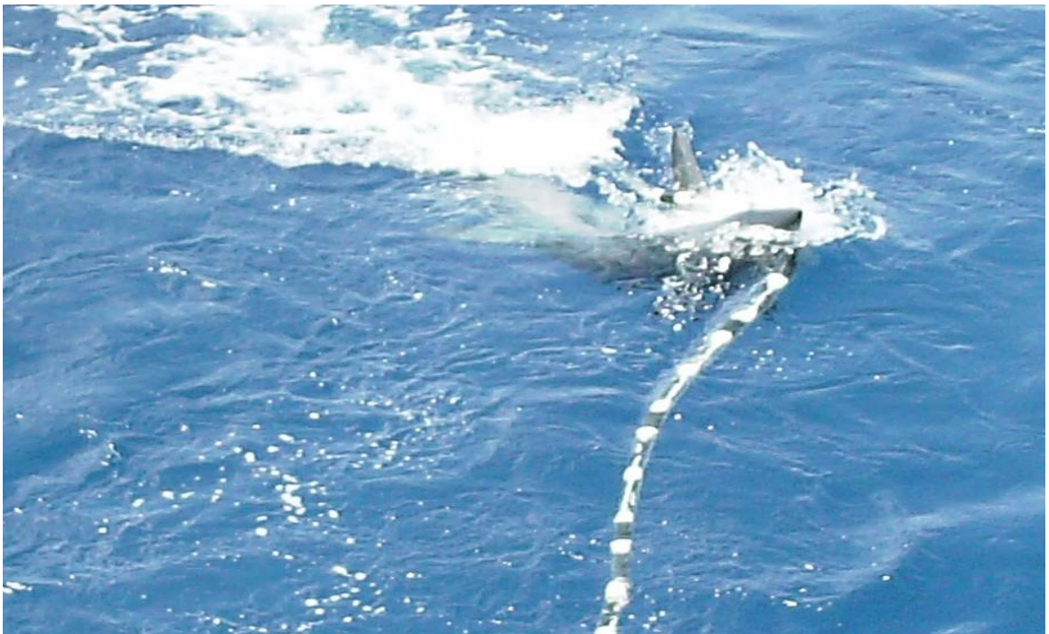
Figure 10: Shark biting the receiver cable (Courtesy of CGG).
