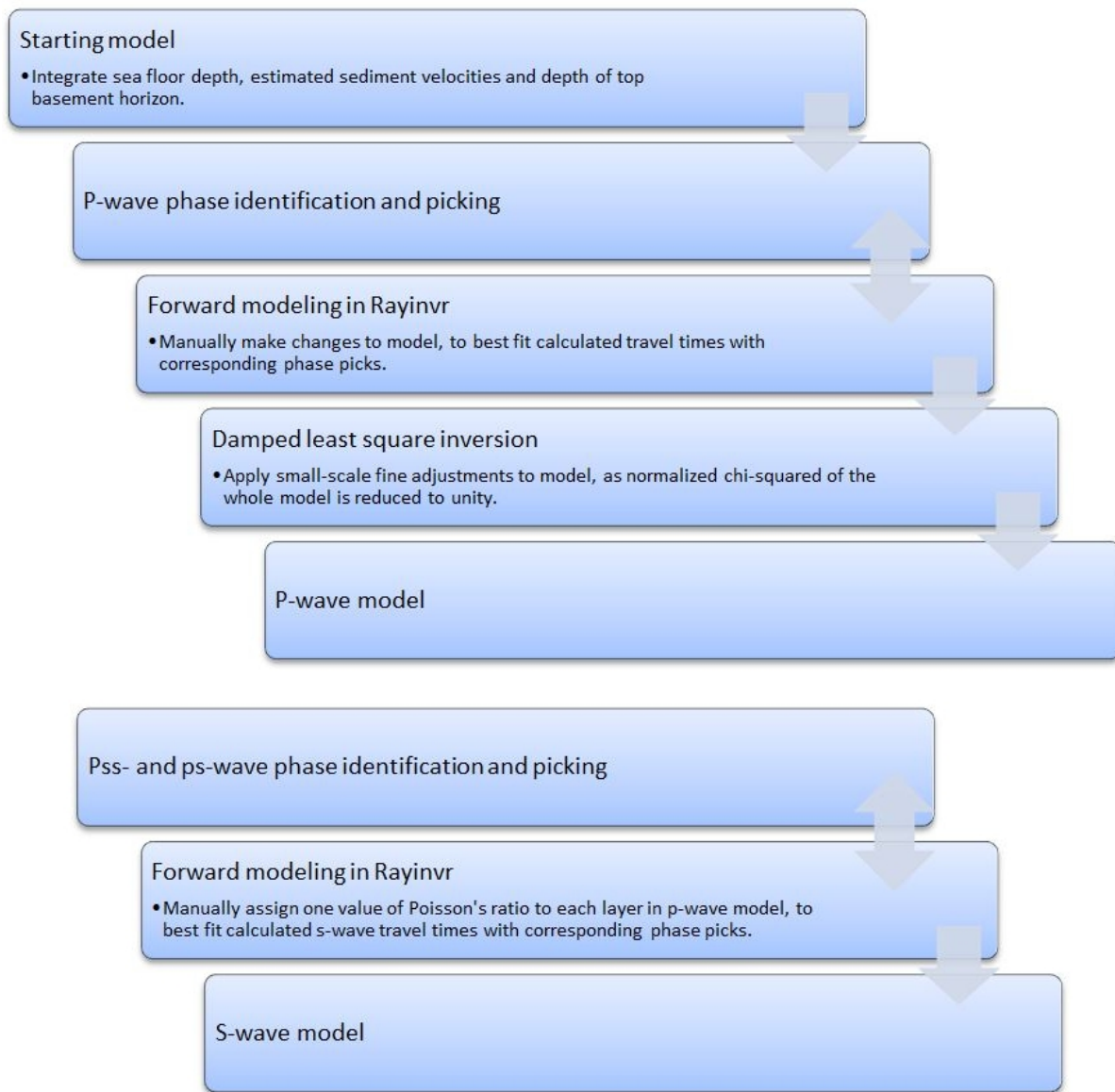
Figure 7.1: Chosen procedure of making velocity model. The two-way arrow tells that despite identification and picking of phases was done first, adjustments was again made after having modeled with Rayinvr. The two steps were repeated numerous times.
