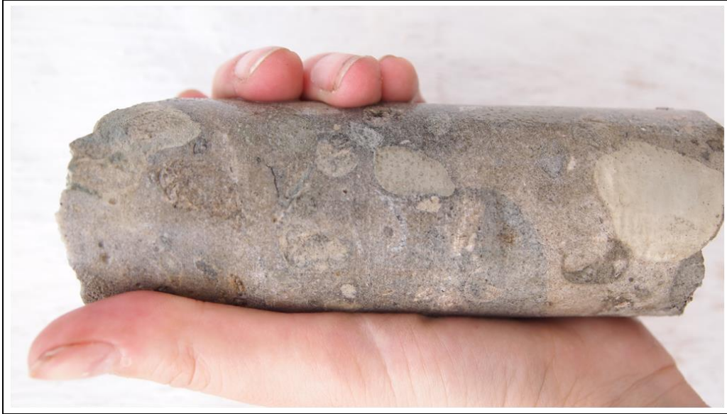
Figure 4.15: Normal graded sandstone of facies F3b, containing rounded clay rip-up clasts and small white shell fragments (core 17, well site 21).
