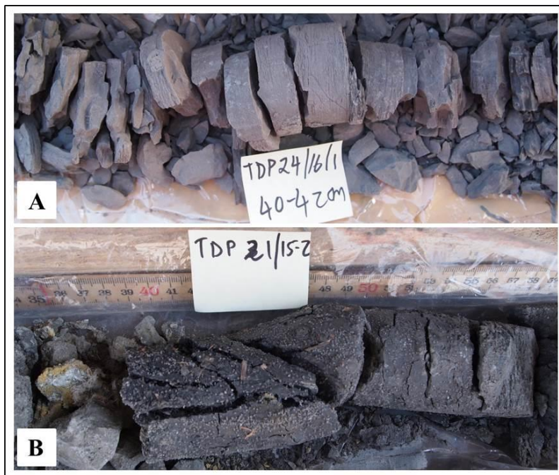
Figure 4.11: A) Greenish/grey slightly laminated claystone of facies F1 (core 16, well site 24). B) Dark grey-black structureless claystone of facies F1 (core 15, well site 21).
