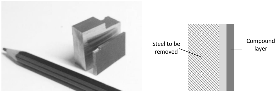
Figure 3-7: To the left a piece of the PPN sample surface after cutting and to the right an illustration of the goal of the thinning process.
