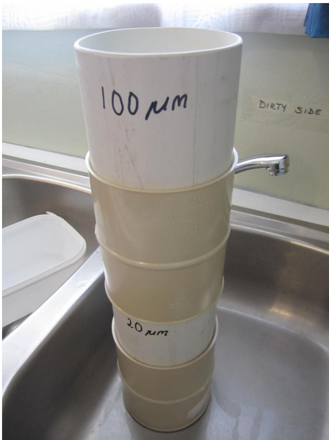
Figure 8 The 100 \mu\text{m} sieve on top of the 20 \mu\text{m} sieve allowing the researcher to use both sieves simultaneously.
