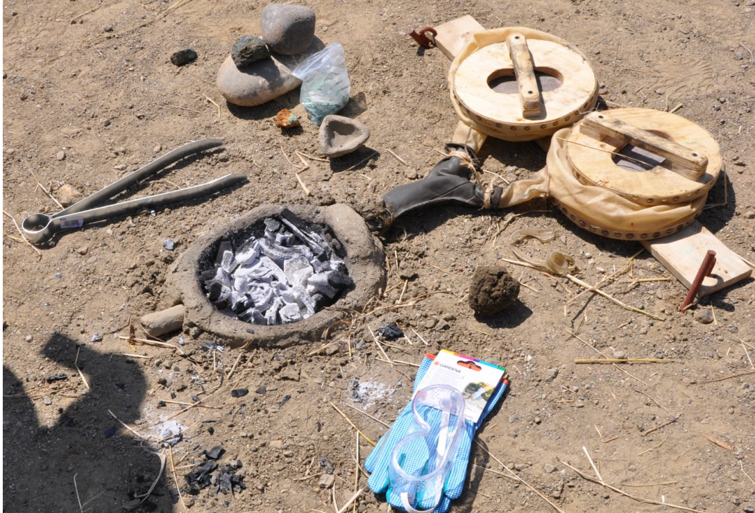
Figure 2: Open furnace of clay, partly buried in soil, with bellows, crucible, iron grips, rocks to crush the ore, ore and burning charcoal in furnace.
