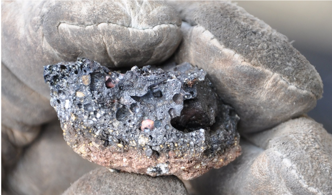
Figure 4: Part of a crucible (lower part) broken to show slag (black upper layer), copper prills forming in the lower slag, as well as holes evacuated by copper prills (lost in breakage of crucible). The crucible shows some damage from the furnace.
