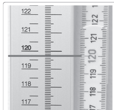
Figure 2 Procedure to determine correction values in the NCG-study. As part of the procedure to determine correction values in the NCG-study, the value of the stadiometer at each school (left) that corresponded to 120.0 cm of the reference length (right) was recorded. In practice, the folding rule was blacked out above and below 120 cm to avoid misunderstanding.
