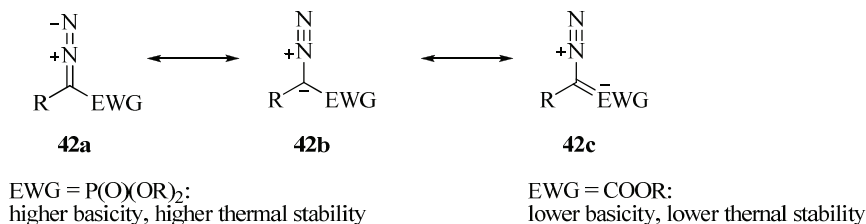
Figure 5.1 Mesomeric structures responsible for basicity and thermal stability of diazo compounds by Jugelt et al. 10
