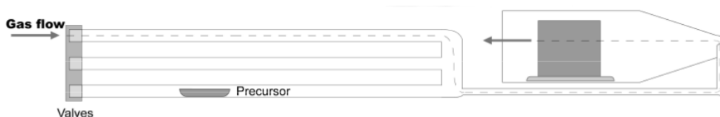
Figure 17: Schematic of the interior of a F-120 Sat ALD reactor. Gas flow arrows indicate gas flow during pulsing of precursors. 15
