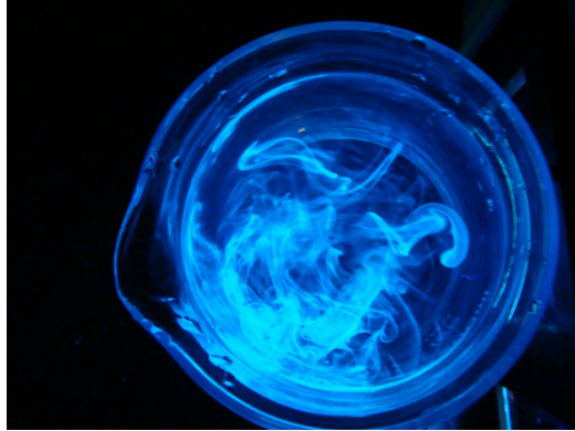
Figure 3: A piece of Lignum Nephriticum dropped into an alkaline solution and illuminated with a UV hand lamp. 6
