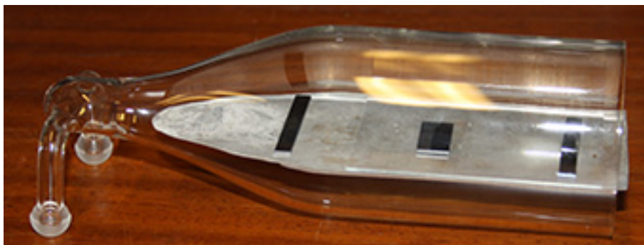
Figure 20: Reaction chamber used in ALD. Gas flow enters the chamber in the to glass tubes pointing down on the left side and exit to the exhaust to the right. Front substrate on the left, back substrate on the right and main substrate in the middle.
