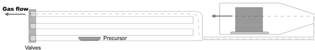
Figure 18: Schematic of the interior of a F-120 Sat ALD reactor. Gas flow arrows indicate gas flow during purging of precursors. Image adapted from Klepper. 15
