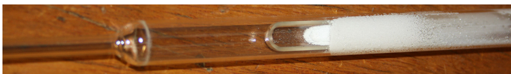
Figure 35: Image of precursor tube with a boat containing precursor. During purging the precursor recrystallizes on the inside of the tube, called back sublimation.
