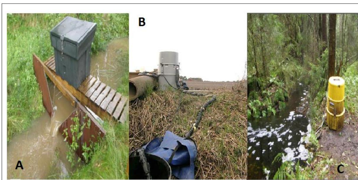
**Figure 7: Autosamplers installed in 2009 at sampling streams. Pictures ‘A and B’ shows the ISCO 6700 autosamplers at Støa1 and Hug respectively while picture ‘C’ shows the Manning autosampler at Dalen. Photo by Prof. Rolf D. Vogt.**
