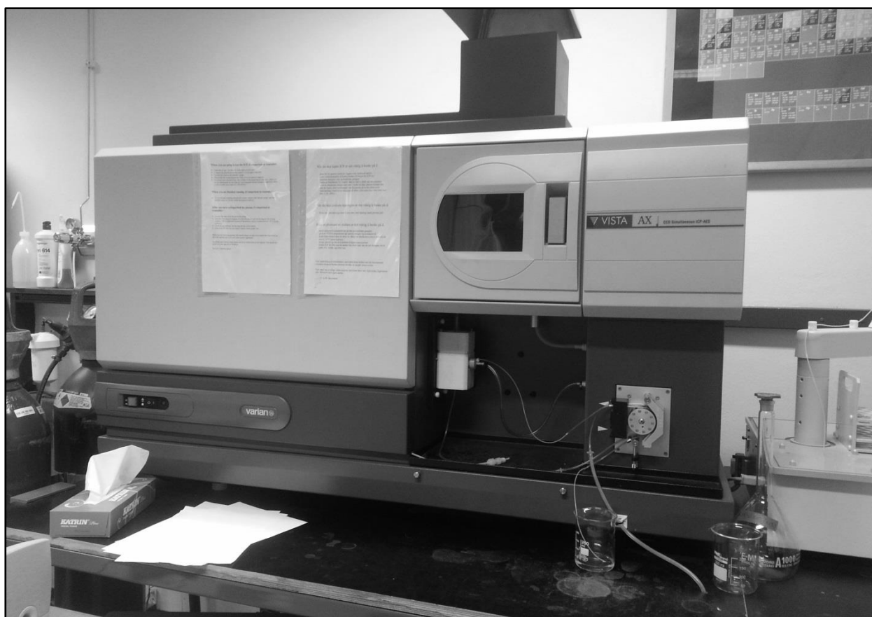
Figure 5 Picture of the ICP-OES instrument used for analysis.
