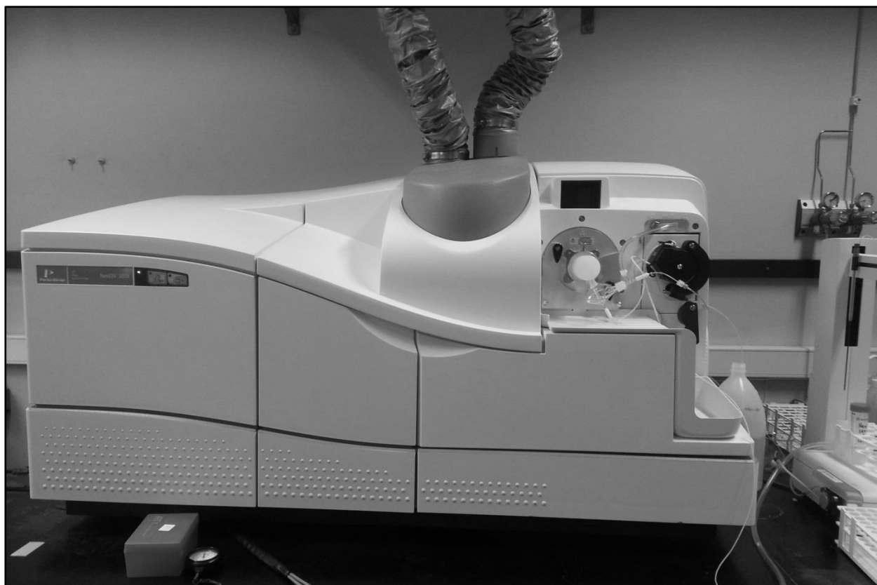
Figure 6 Picture of the ICP-MS instrument used for analysis.
