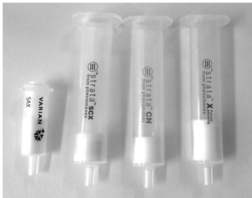
Figure 3 The SPE cartridges used, showing SAX, SCX, CN and RP, from left to right.
