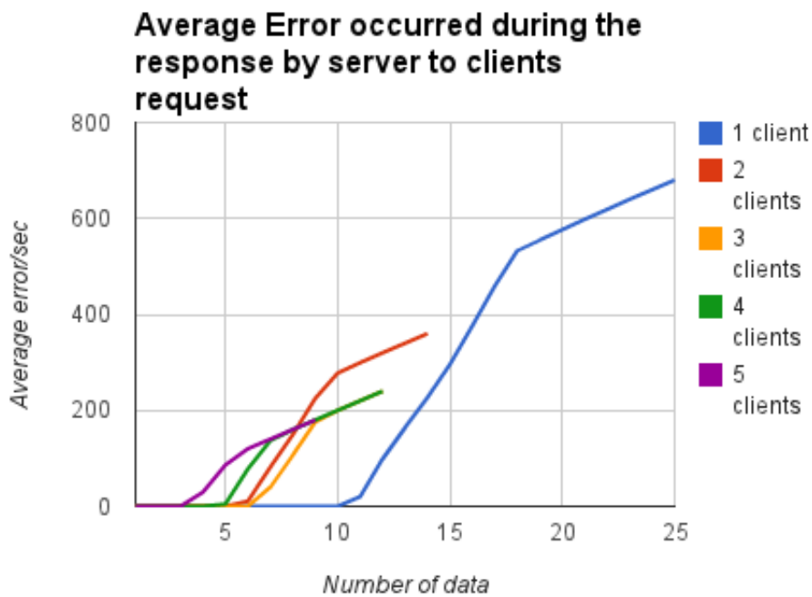
Figure 3.10: The average error occurred during course of reply sent by server to clients requests.
