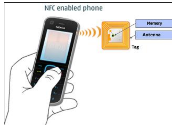
Figure 12: Internal structure of NFC tag 11
