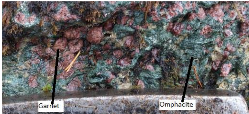
Figure 2 - Typical eclogite minerals from Engebøfjellet. Grain size in the rock is larger than in typical eclogite at Engebøfjellet. Hammer head as scale.
