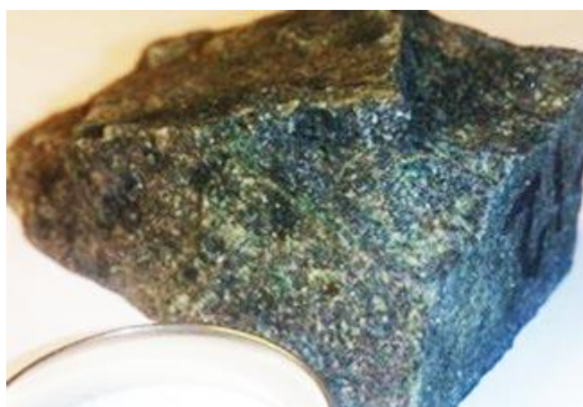
Figure 96 – Hand specimen from SK-30. Sample appears to be amphibolite, but turned out to be fresh eclogite.
