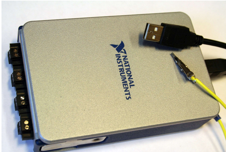
Figure 5.4: The DAQ car used, a NI9223 Analogue Input Module and a 1-slot NI CompactDAQ chassis with USB connection. Left is connection panel for inputs. To the right is USB plug for PC connection and wire for ground connection.
