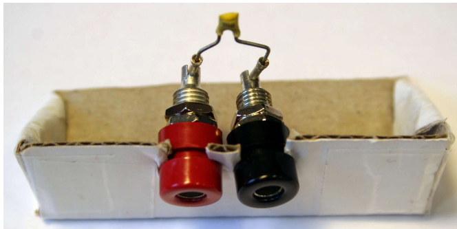
Figure 5.9: Model dock constructed of cardboard and two banana plug connectors. Ceramic capacitor mounted for measurement.
