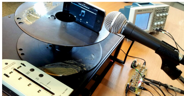
Figure 5.16: Equipment setup for testing the TFS. Seen in the picture is the sound pressure level measurement instrument, sound source (iPhone 4), microphone, oscilloscope and of course the frequency shifter PT4.1.
