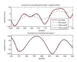
Figure 6: Excerpts from Take 1 and Take 2. While a 5 Hz filter cutoff works well for the Take 2 below, the rapid motion needs a 10 Hz or a 15 Hz cutoff frequency to follow the details in the recording.
