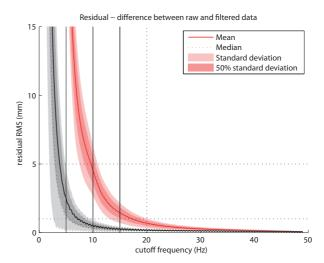
Figure 5: Statistical results of the *residual analysis* of the recorded data. Take 1 (rapid motion) is in red while take 2 is given in black.
