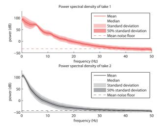
Figure 4: PSD estimation of the recorded data using Welch's method. The data is shown as statistical results of all 20 recordings, with results from both Take 1 (rapid) and Take 2.
