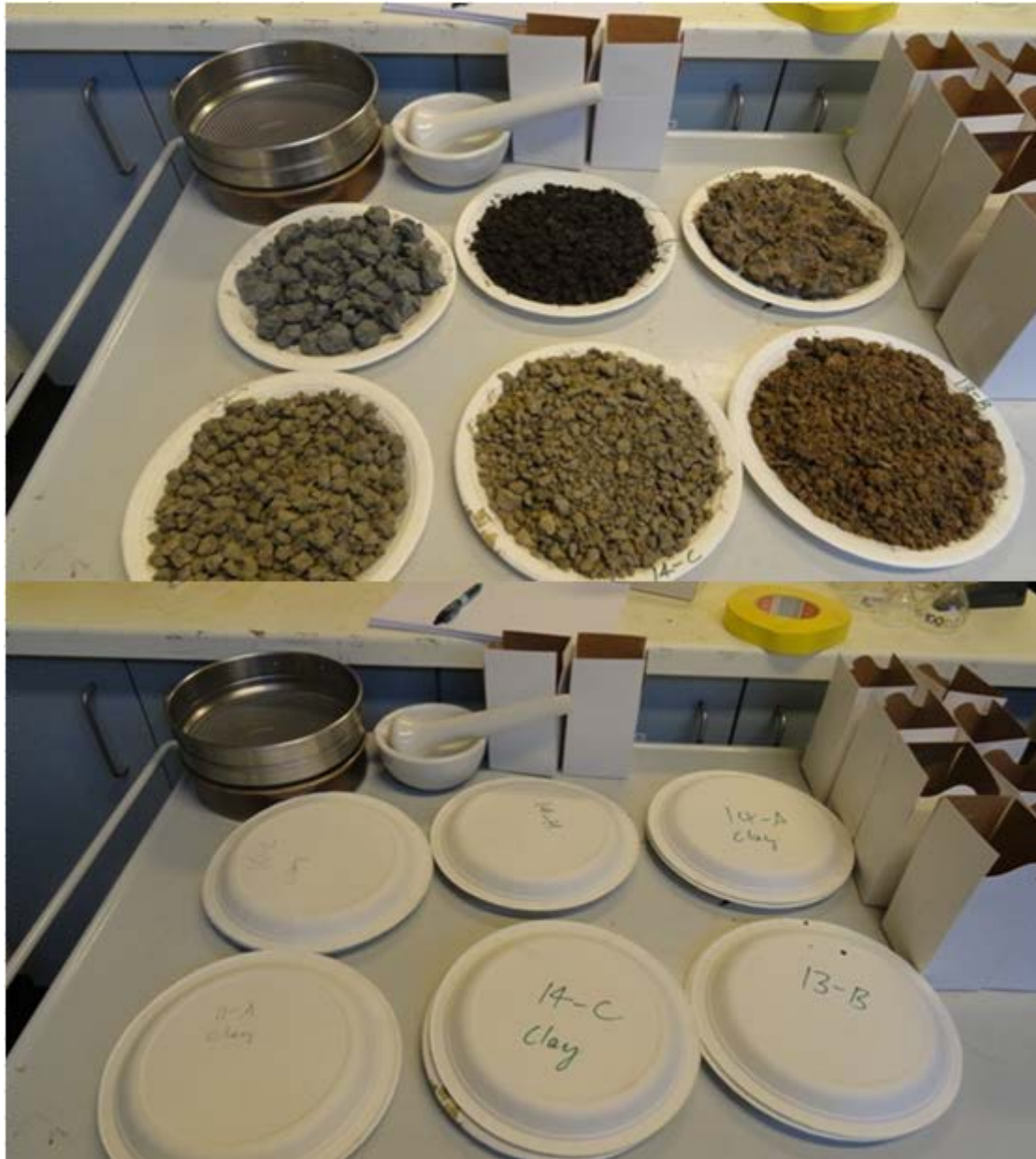
Figure 19: Drying of soil samples from various soil types and horizons (upper panel). During the drying the samples were covered as shown in the lower panel.
