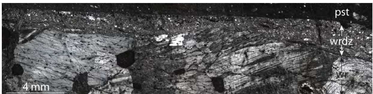
(e) Photomerged micrographs of the lower part of the pst in HK4, the fine grained wall-rock damage zone and the fractured plag in the wall-rock related to it. Note the variable thickness of the wall-rock damage zone. (HK4, xpl).
