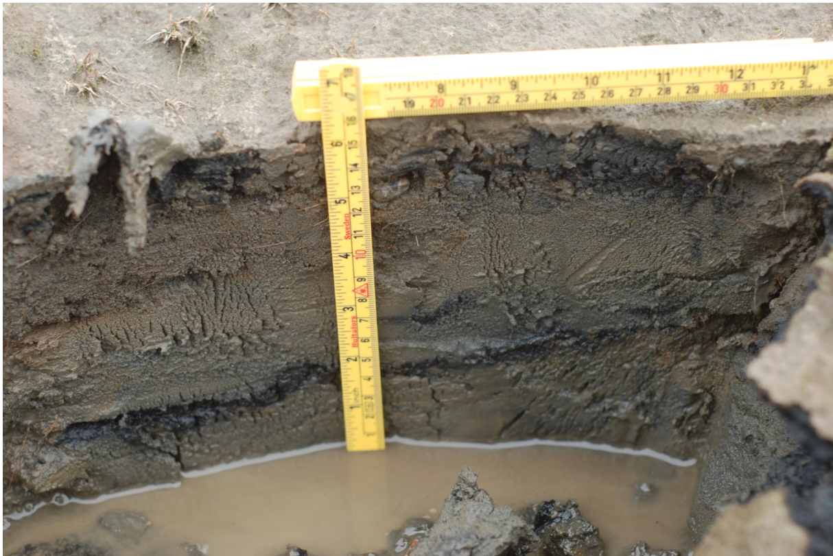
Figure 50: Picture from profile P1 showing heterolithic bedding and rootlets, which can be indicating flood-plain, as the upper part of a point-bar deposit.
