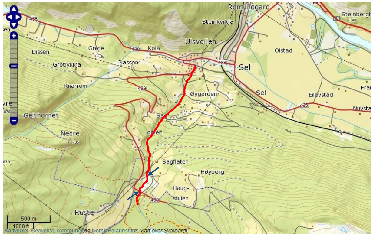
Figure 1.3 The study area map of the Sagdalen debris flow occurred in 10 th June 2011, red curve shows the track of the debris flow, and the two pots pointed by the blue arrows represented the destroyed bridges, taken from www.norgeskart.no .
