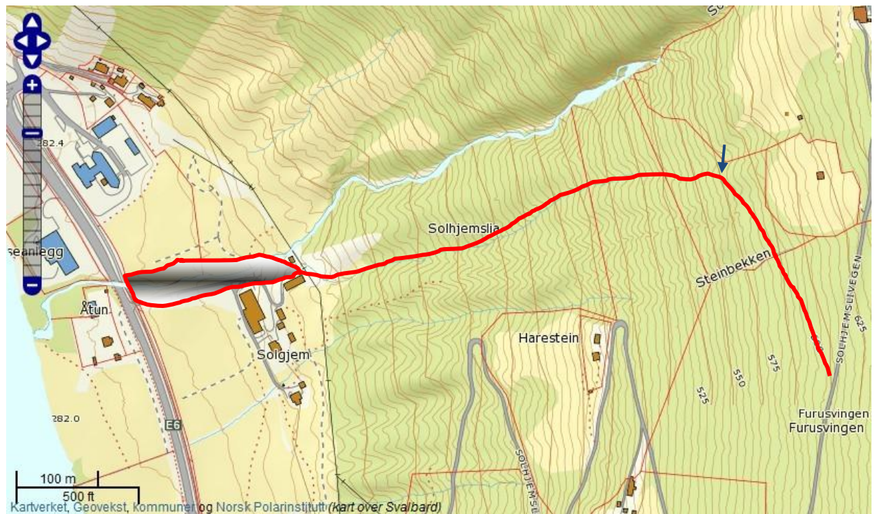
Figure 1.2 The study area map of the Solhjem debris flow occurred in 10 th June 2011. Red curve shows the track of the debris flow, and the gray shadow represents the deposition zone, taken from www.norgeskart.no . The pot pointed by the blue arrow was the failure point of the slope.
