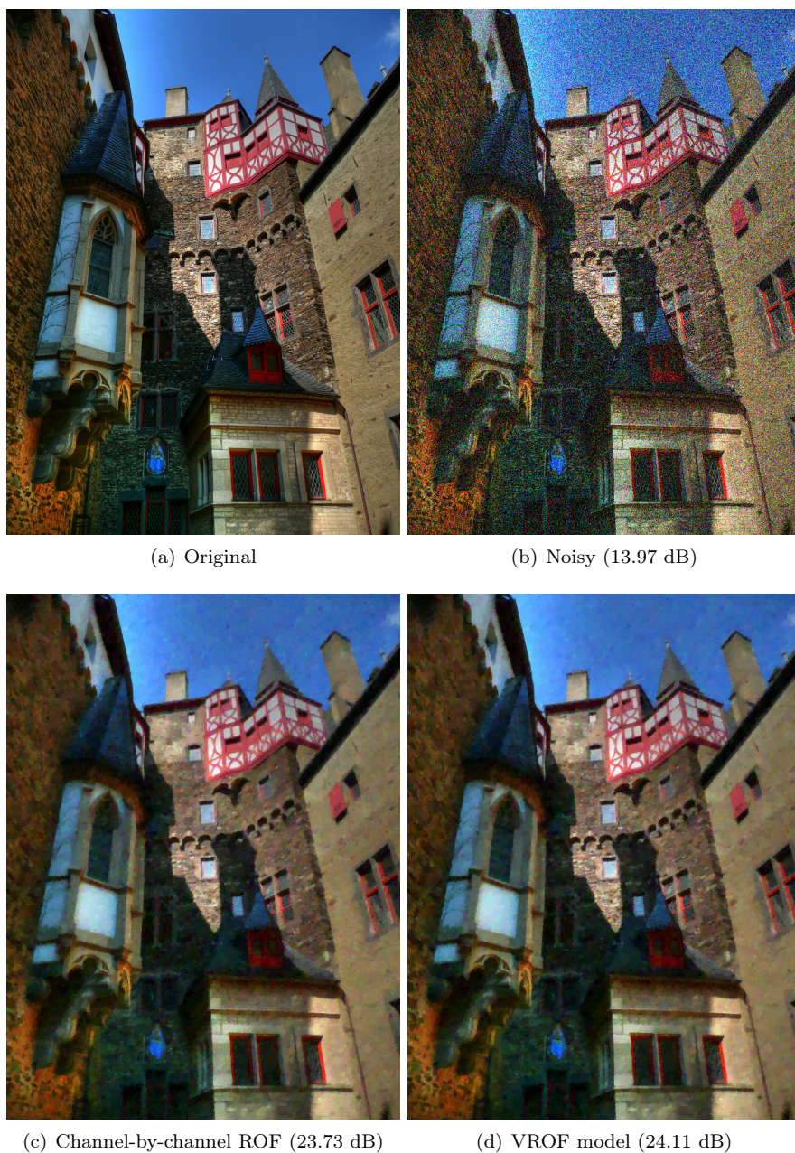
FIGURE 6.3: Denoising colour images. The first row displays the original and noisy colour image. The noise is additive white Gaussian with a standard deviation of \sigma = 0.2 . Below are the respective denoising results that come from applying the ROF model separately to each colour channel with \lambda = 6 , and from applying the VROF model with \lambda = 4.1 to denoise the colour channels jointly. The PSNR is displayed below each restored image.
