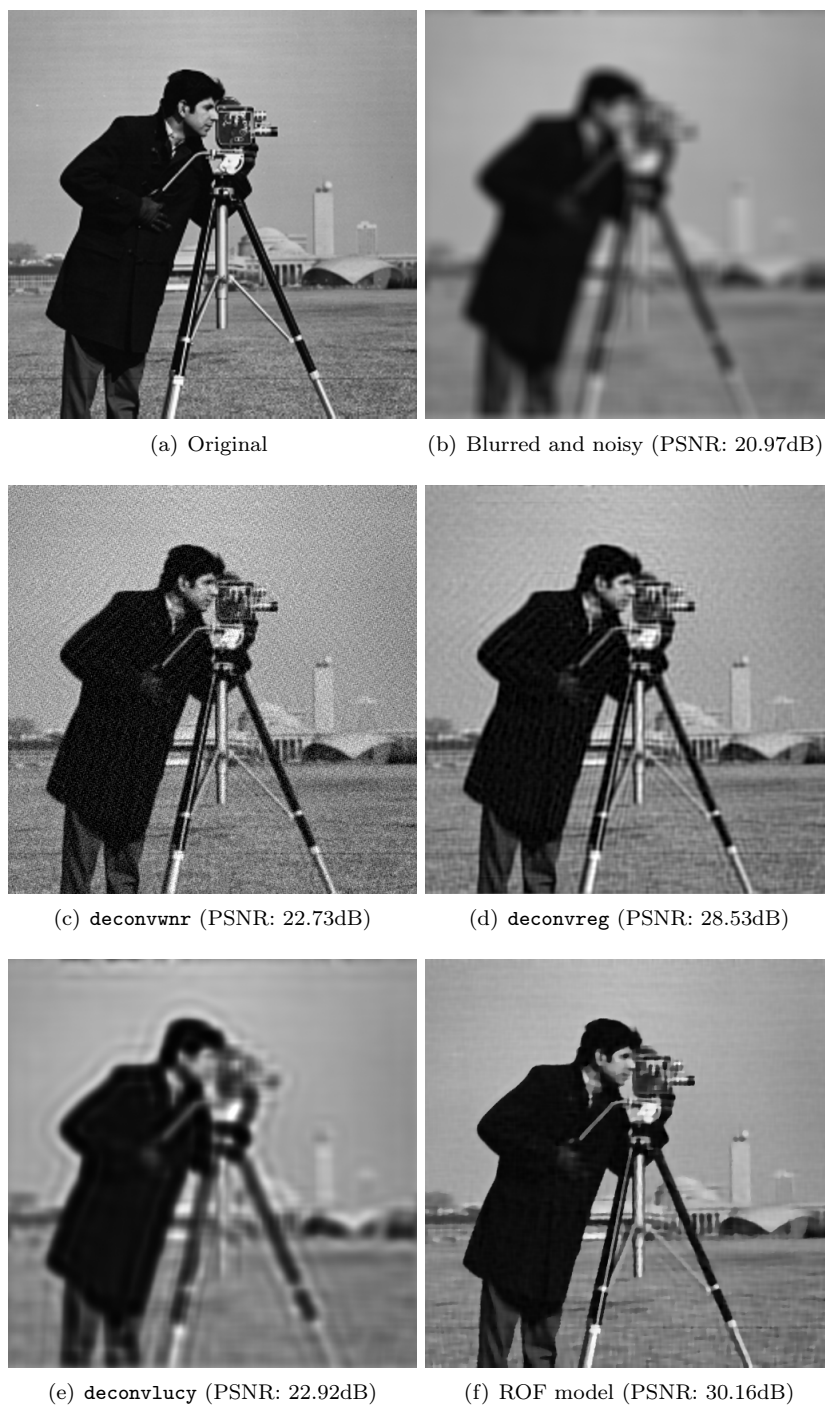
FIGURE 6.4: Image deblurring. The original image (a) is blurred by a Gaussian PSF (6.4) with c = 11 , and white Gaussian noise with a standard deviation \sigma = 10^{-3} is added to produce the image in (b). The subsequent images show the restoration with (c) deconvwnr , (d) deconvreg , (e) deconvlucy , and (f) the ROF model.
