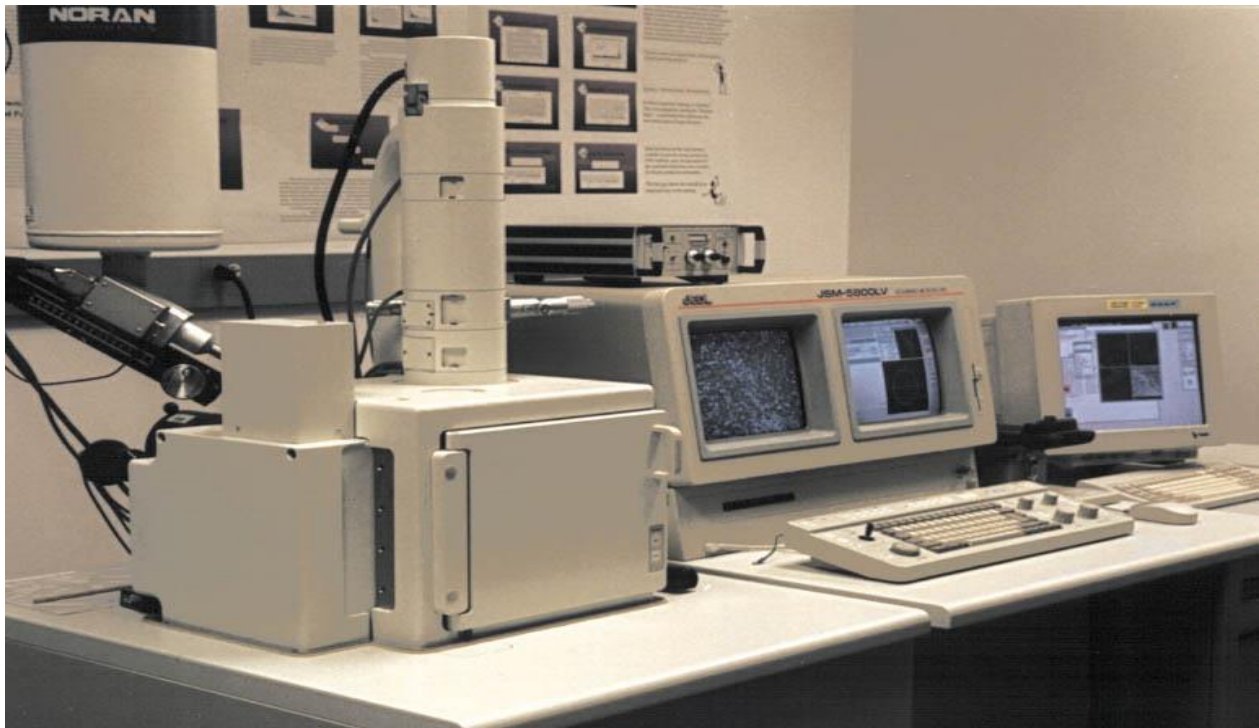
Figure 2.1: A typical representation of SEM instrument, showing the electron column, sample chamber, EDS detector, electronics console, and visual display monitors (adopted from Swapp, 2012).
