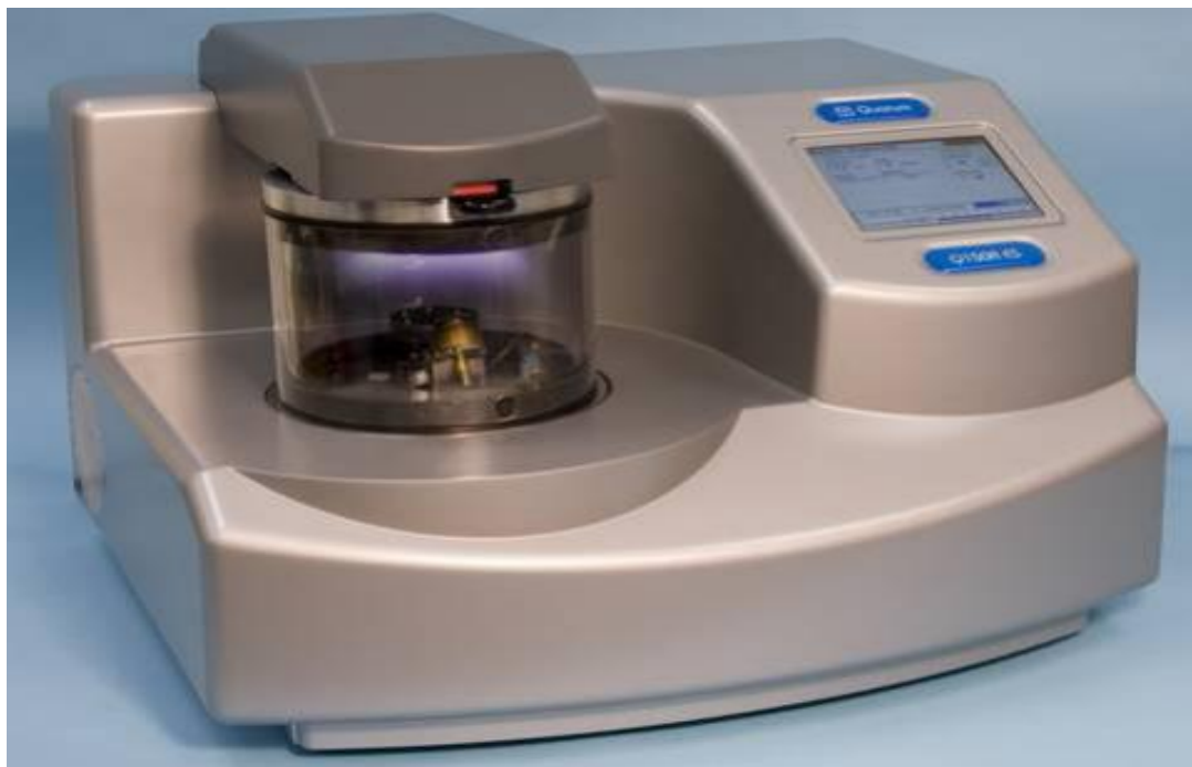
Figure 2.2: View of Quorum Sputter Coater (Q150R S/E/ES) a Sample Preparation Instrument (adopted from QUORUM, 2013).
