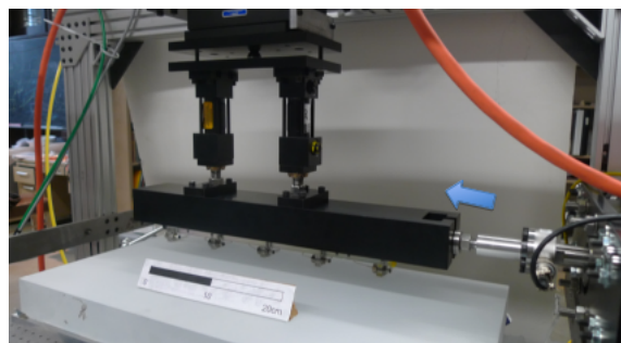
Figure 3.8: A picture of how the shear load is applied to the system. Photographed by J.Trømborg
