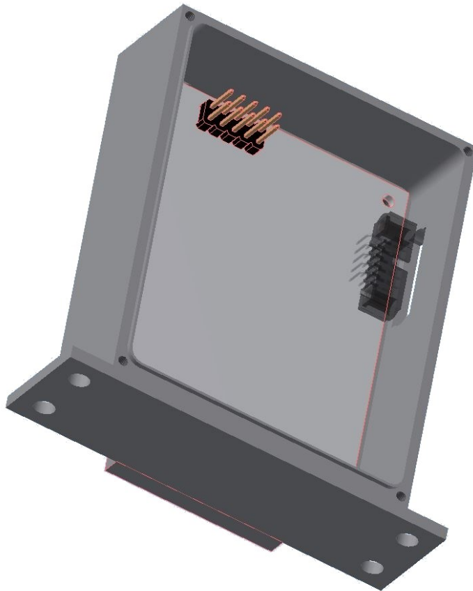
Figure 5.2: Rear view of the DSS2 enclosure.
