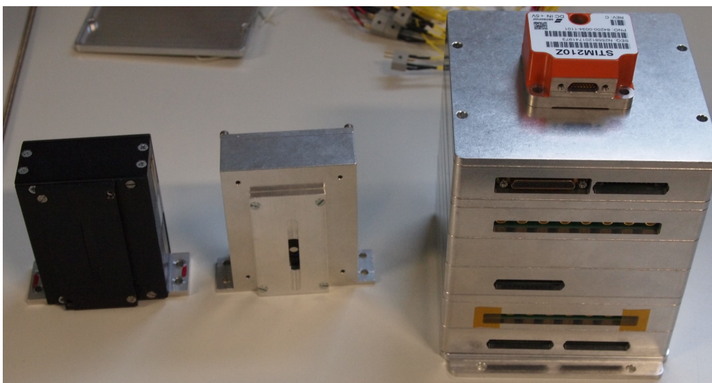
Figure 6.14: The complete UiO-stack with the STIM210 on top and the sun sensors, both the DSS and the DSS2.
