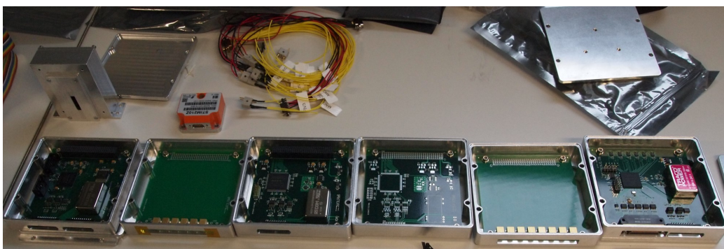
Figure 6.15: All the DAQ-boards for the UiO instruments, the DSS2 and STIM210 units.
