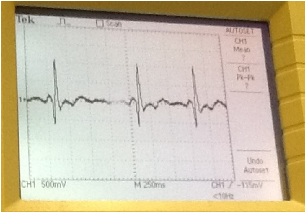
Figure 7.3: ECG Wave from the output of the ECG PCB
