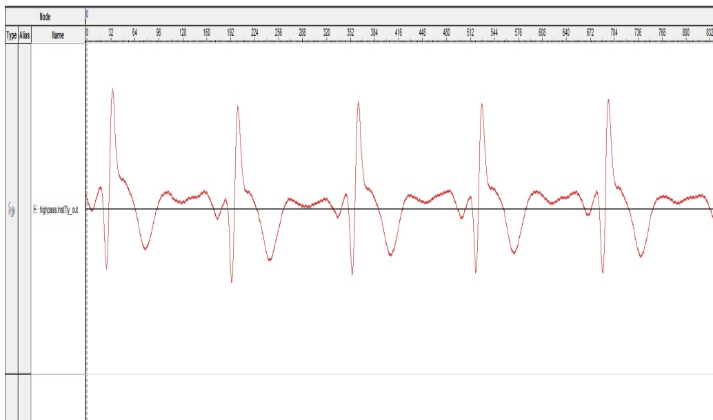
Figure 7.8: Output of the highpass filter
