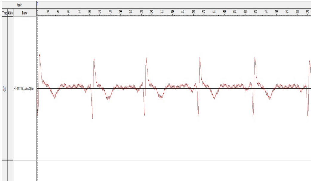
Figure 7.6: ECG wave at the ADC output The ECG signal at the output of the ADC. The 50 Hz interference is noticeable.
