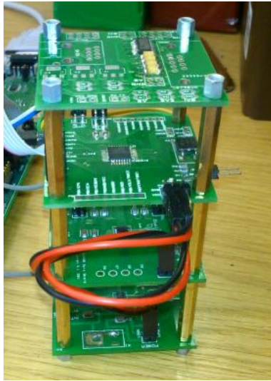
Figure 16: Sensors, micro-controller, and power and serial board stacked together.
