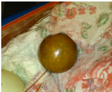
Figure 59: Copper acoustic target used in the field test.
