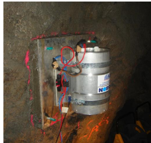
Figure 3.5: Photograph of the electrodynamic shaker mounted to the rock wall at the Oslofjord site.
