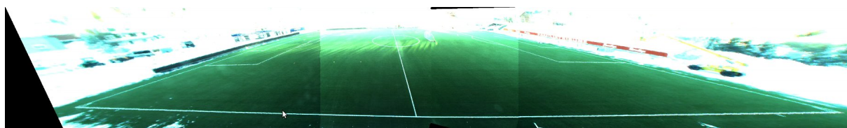
Figure 3.26: Panorama image warped using matrices generated by our calibration tool
