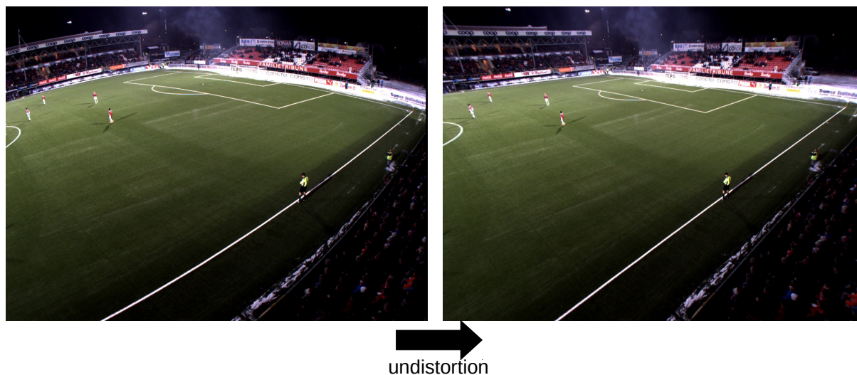
Figure 2.5: Fixing barrel distortion. Note the distorted lines in the left image
