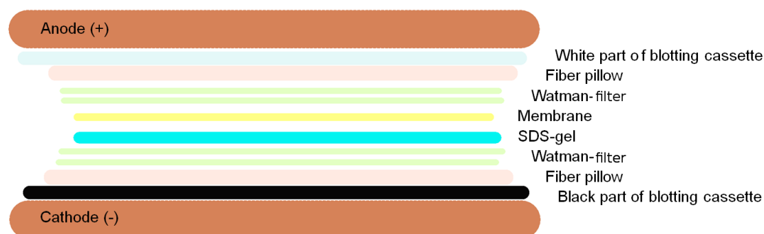
Figure 3.4: Western blotting cassette. The blotting cassette is stacked in the order from cathode to anode; black part of blotting cassette, fiber pillow, 2x Watman-filter, SDS-gel, membrane, 2x Watman-filter, fiber pillow, white part of blotting cassette.
