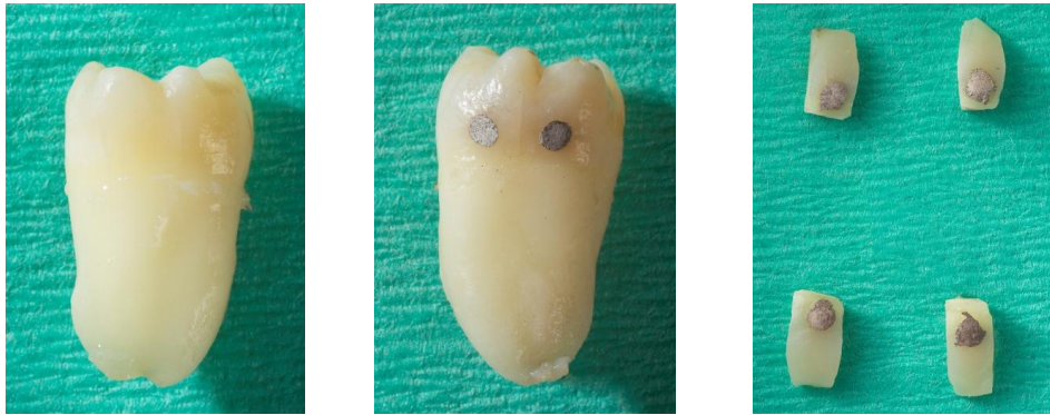
Figure 13. Amalgam fillings (approximately 1 mm in diameter) were made in human third molars about 2 mm above the enamel-cement junction for use as reference surfaces. One specimen included one amalgam filling [Hove, 2008].
