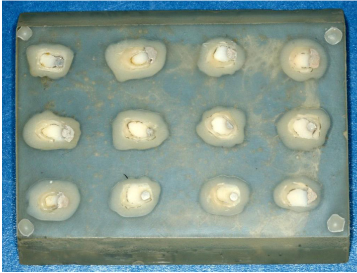
Figure 14. The enamel specimens with amalgam reference surfaces were mounted in epoxy resin blocks (Epofix ®, Struers, Denmark) ( Study 1, 2 and 4 ). The specimens were ground flat in Study 1 and 4 , but kept natural in Study 2 .
