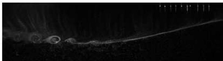
Figure 2: Composite image (side view) of breaking internal solitary wave approaching probe assembly (top right)
