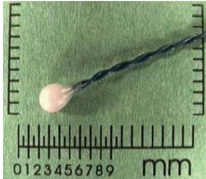
Figure 3. Ultrasonic crystal (courtesy of Sonometrics Corp., London, Ontario, Canada). Sonomicrometry is the measurement of distances between transmitting and receiving ultrasonic crystals (piezoelectric ceramic crystals) by using the speed of sound principle. Having transmitter as well as receiver capabilities, the 2 mm diameter crystal transmits ultrasound bursts (travelling at 1540 m/s in soft tissue), which are being received by another crystal. The elapsed time from transmission to reception is a direct and linear representation of the spatial distance between the crystals. Wires leading from the crystals are connected to a digital sonomicrometer (Sonometrics Corp.), which is able to transmit from a single crystal to multiple receiving crystals, and thus rendering multiple distances per ultrasound burst. Transit time is measured in steps of 15 nanoseconds, resulting in a spatial resolution of 0.024 mm.
