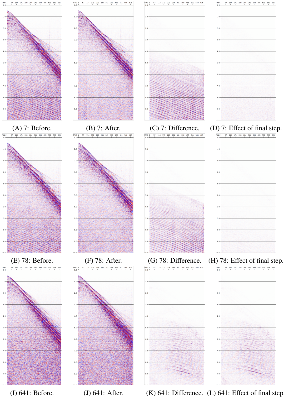
Figure 5.11: Before (first column), after (second column) and difference plot (third column) for shot 7, 78 and 641 after applying the VF method and \tau - p muting followed by the \tau - p to common- p method. Fourth column show the effect of the final \tau - p to common- p method on the shot gathers.
