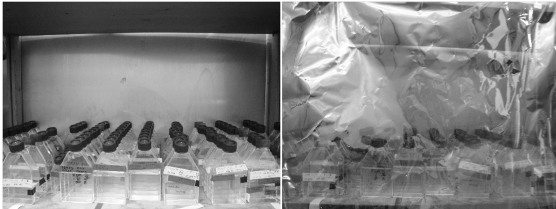
Figure. 5 Cultures of Daphnia during the reciprocal experiment. Animals were kept in the culture bottles that were randomly distributed and covered by foil (right). Animals were placed in a temperature-controlled room, at 20 °C.
