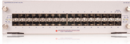
Figure 2.1: Using specialized hardware is preferable for high bandwidth testing. This hardware module from Spirent is created to be able to fully saturate high performance Ethernet network devices to their maximum capacity. HyperMetrics dX 32-port 10G Ethernet test module [image online] Available at: http://www.spirent.com/Solutions-Directory/Spirent-TestCenter/HyperMetrics_dX [Accessed 1 March 2012]
