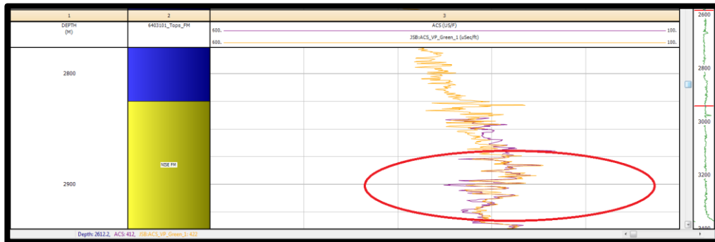
FIGURE 3. 2 - GREENBERG-CASTAGNA DERIVED CURVE (ORANGE) AND REAL DATA (PURPLE). THEY MATCH IN THE ELLIPSE.
