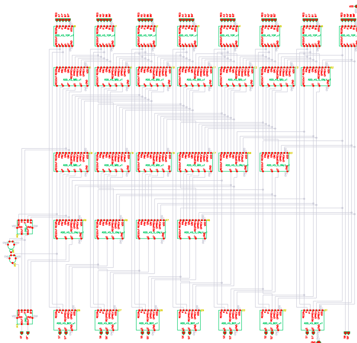
Figure 3.8: Schematic of a DCVSL 8-bit Kogge-Stone adder with overflow output.
