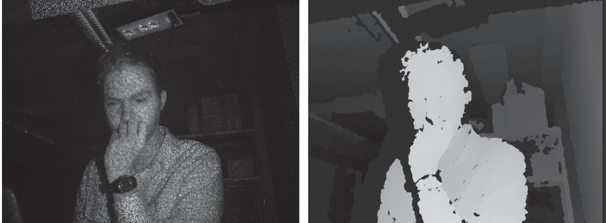
(a) Illustration of the structured light technique performed by the Kinect (b) The resulting depth map produced by the Kinect sensor
