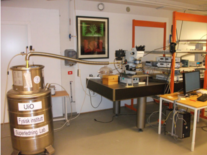
Figure 2.4: The setup with the helium flow cryostat.
