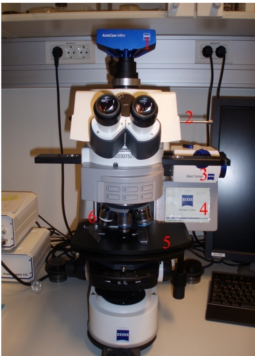
Figure 1. Some of the components of the fluorescence microscope 1. Camera. 2. Plunger that controls the light path. 3. ApoTome. 4. Touch screen. 5. Sample platform. 6. Objectives.
