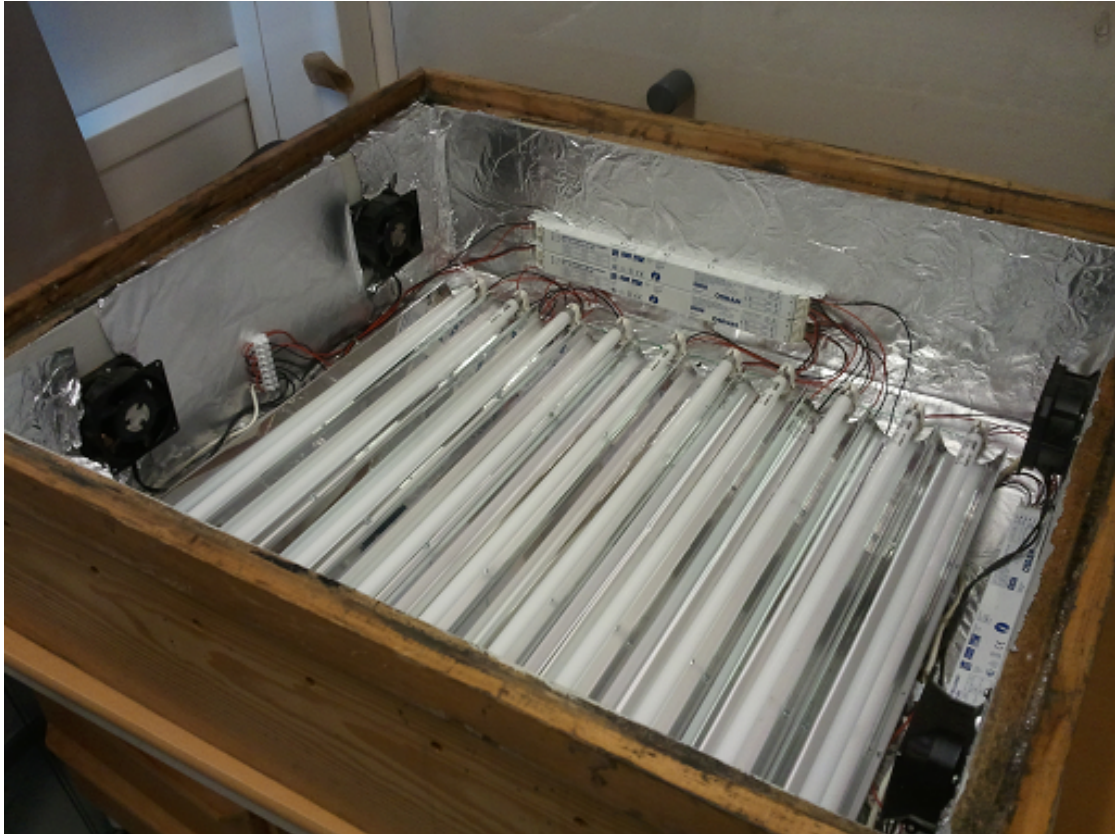
Figure 3.12: The lightbox is displayed with its interior. The surface is placed as a lid on the top of the box.
