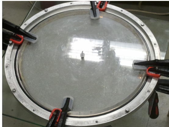
Figure 3.40: The assembled deformable porous sample structure. There is a trench between the sample plate and the sample holder frame, which is called the fill trench
