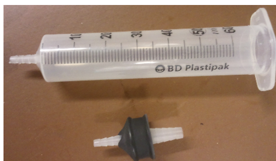
Figure 3.41: The beadinjector shown with its removable air inlet, the replaced syringe tip is a two-way connector which is cut in half.
