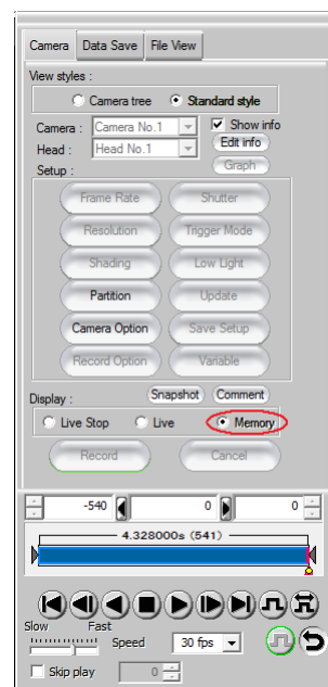
Figure 3.27: The "Memory" mode of the display shown in the control panel.
