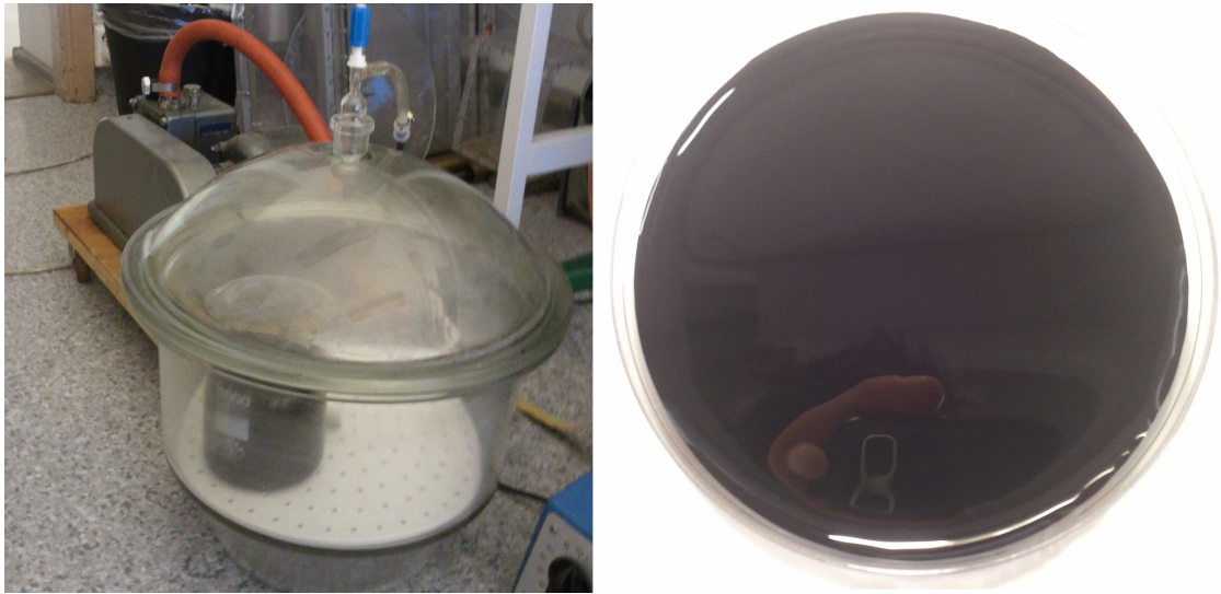
Figure 3.7: Left: The vacuum excitator containing a sample and connected to the vacuum pump. Right: An "acid black 2" sample of aqueous glycerol.
