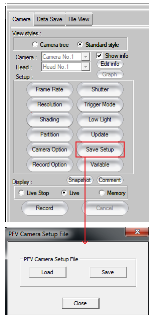
Figure 3.23: The "Save Setup" option in the control panel.
