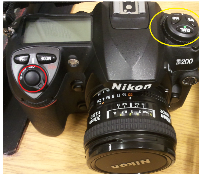
Figure 3.30: The D200 with the shutter release button indicated with a red circle and the mode dial indicated by a yellow circle.
