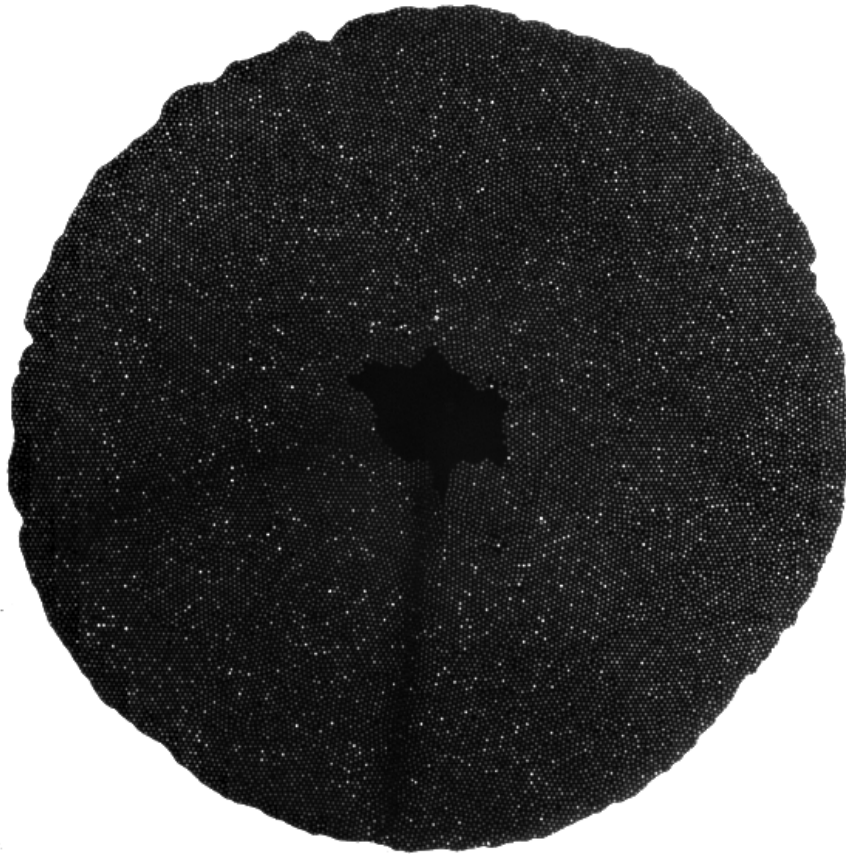
Figure 2.12: A stable viscous displacement of air (white) by a viscous liquid (black) in a deformable two dimensional porous media. Note that the displacement front is still within the porous media which is invisible while saturated with air.
