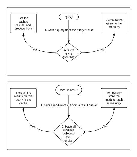
Figure 6.1: Caching functionality in the Query Broker
