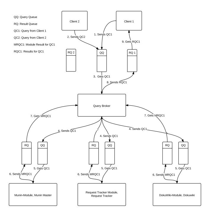
Figure 5.1: Prototype Information Flow
