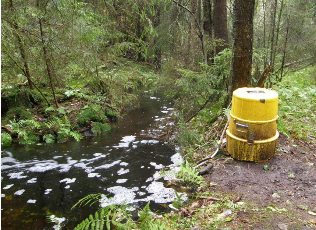
Figure 20: Auto sampler installed at sampling site of the Dalen (Photo taken by Rolf D. Vogt 29.08.11).
